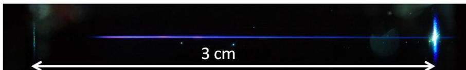
**Figure 4.** Side photography of the blue fluorescence of  $\text{SiO}_2$  induced by a self-guided laser pulse at 1.9  $\mu\text{m}$  with  $P = 30 \text{ Pcr}$ . The laser pulse is focused on a 70  $\mu\text{m}$  spot (FWHM) at the left surface of the 3 cm thick sample.
