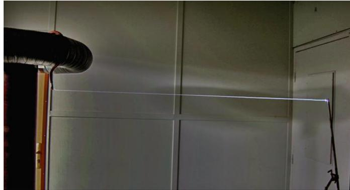
**Figure 19.** Photography of a Tesla guided discharge of 1.7 m.
