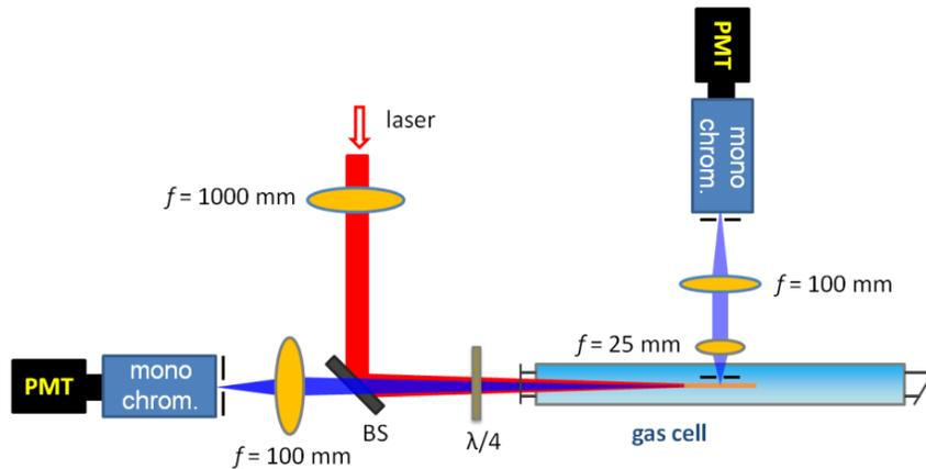
Fig. 1. Schematic experimental setup. The incident femtosecond pulse is focused by an  $f = 1000 \text{ mm}$  lens. The dichromatic beam splitter (BS) steers the 800 nm pulses inside the gas cell filled with Nitrogen gas or its mixture with air. The backward radiation from the plasma is collected by a  $f = 100 \text{ mm}$  fused silica lens into the slit of a monochromator. The signal is measured with a photomultiplier tube (PMT).
