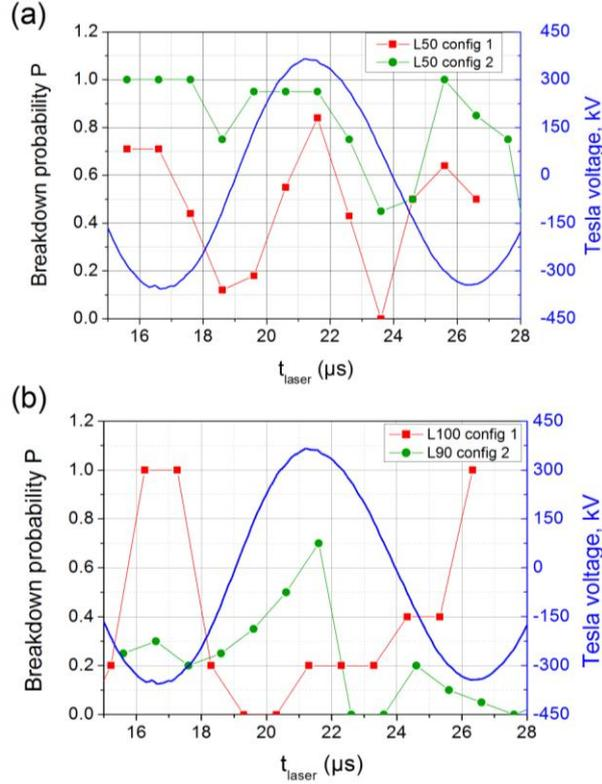
FIG. 4. Evolution of the breakdown probability  $P$  with  $t_{\text{laser}}$ . (a):  $L = 50$  cm, configuration 1 (red solid curve and squares) and configuration 2 (green solid curve and circles). (b)  $L = 100$  cm, configuration 1 (red solid curve and squares) and  $L = 90$  cm, configuration 2 (green solid curve and circles).
