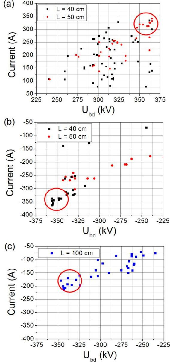
FIG 7.  $(I_{max}, U_{bd})$  characteristics for  $L = 40$  and  $50$  cm. (a): positive quadrant. (b): negative quadrant. (c) Negative quadrant of the  $(I_{max}, U_{bd})$  characteristic for  $L = 100$  cm.
