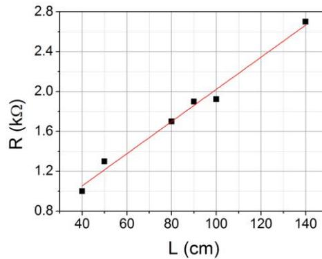
FIG. 8. Evolution of the operational resistance  $R$  with the gap length  $L$  (scatter plot) and linear fit (red solid line). Only breakdown occurring in the voltage range  $-360 \text{ kV} < U_{bd} < -300 \text{ kV}$  were taken into account.
