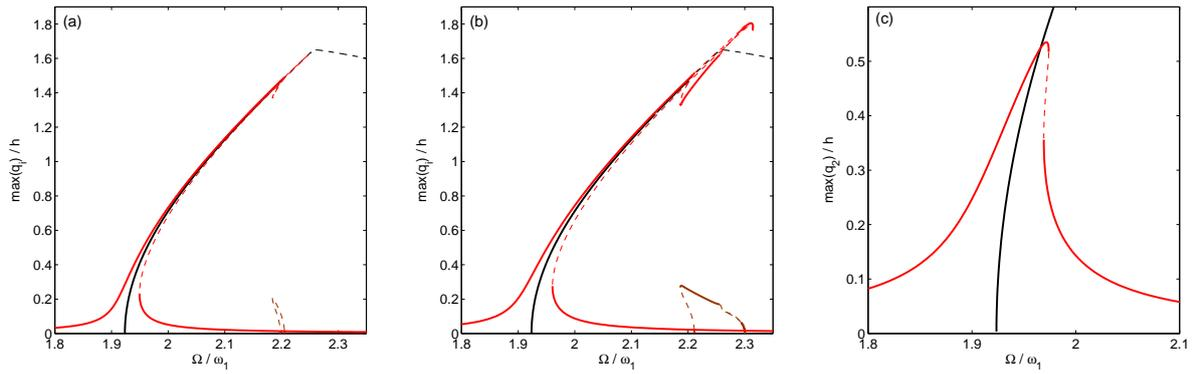
**Fig. 9** Examples of forced-damped vibrations around the NNM for mode 2. (a):  $f = 1.2$  N,  $\chi = 0.001$ ; (b):  $f = 2.0$  N,  $\chi = 0.001$ ; (c):  $f = 3.2$  N,  $\chi = 0.01$ . Mode 2: red, Mode 5: brown.
