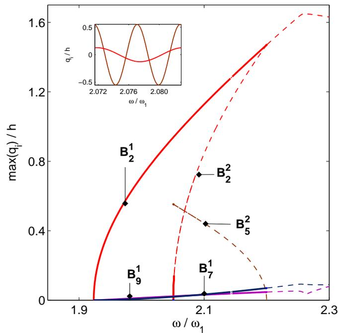
**Fig. 8** Backbone for mode 2 obtained when  $N_w = 16$ . Modes 7 (pink) and 9 (dark blue) are activated by the nonresonant coupling within the SA family; mode 5 (brown) from the AA family is activated by 1:2 internal resonance (see inset).
