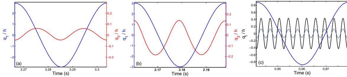
**Fig. 4** (a): Modes 1 (blue) and 2 (red) along  $\mathbf{B}^2$  displaying 1:2 internal resonance. (b): Modes 1 (blue) and 2 (red) along  $\mathbf{B}^3$  displaying 1:2 internal resonance. (c): Modes 1 (blue), 14 (grey) and 16 (black) along  $\mathbf{B}^3$  displaying 1:10 internal resonance.
