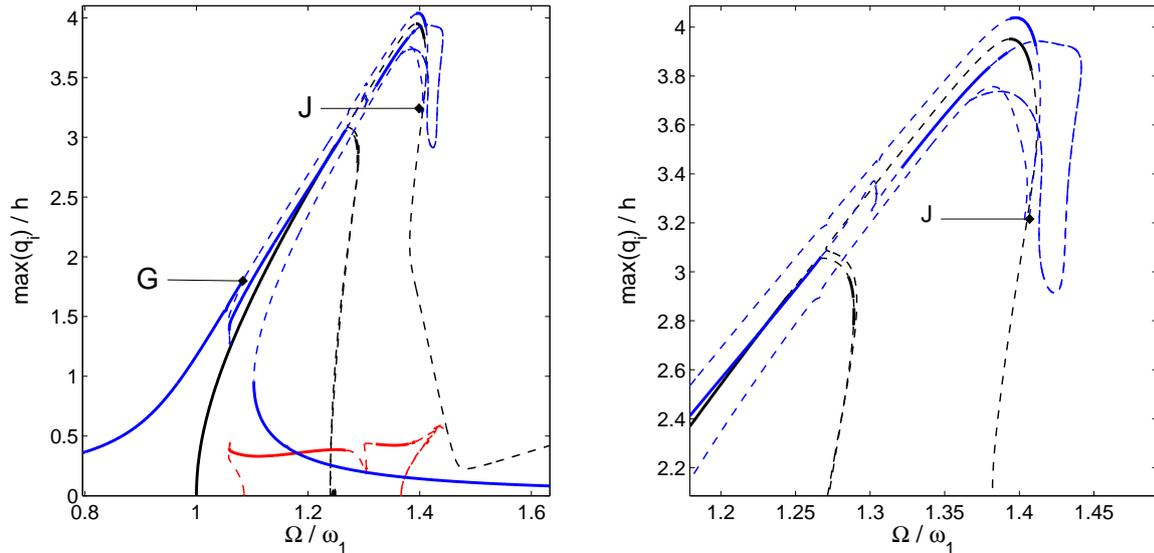
**Fig. 7** Forced response for mode 1 with  $f = 1.36$  N,  $\chi = 0.001$ . **G**: pitchfork bifurcation point leading to the coupled solution; **J** turning point. Mode 1: blue, Mode 2: red.
