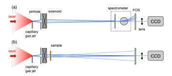
FIG. 1: (a) Experimental set-up for electron beam characterization with an electron spectrometer.
