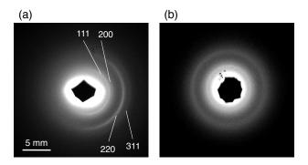
FIG. 3: Electron diffraction patterns from a 10 nm thick polycrystalline Al foil. (a) The diffraction pattern is assymetric because of a spatial chirp in the electron beam. (b) Symmetric diffraction pattern obtained by removing the spatial chirp on the electron beam.
