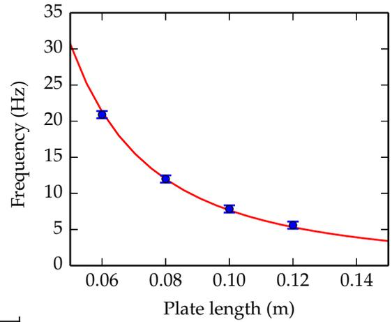
**FIGURE 4.** Mechanical characterization of the plate in a clamped-free configuration. Blue dots: experimental points, red line: theoretical values obtained with manufacturer's values of the plate's characteristics.
