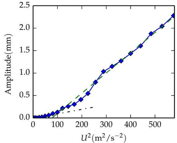
**FIGURE 7.** Evolution of the amplitude of deflection with flow velocity. Blue diamonds: experimental values. Black dash dotted line: linear regression at low flow velocities. Green dashed line: linear regression after divergence.
