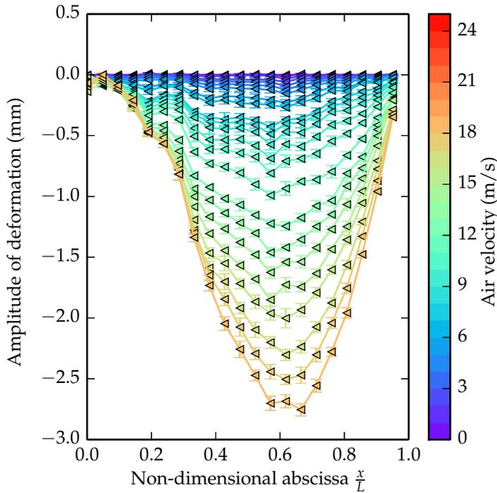
**FIGURE 6.** Profiles of the plate under axial flow for air velocities from 0 to 25 m/s (blue to red lines)
