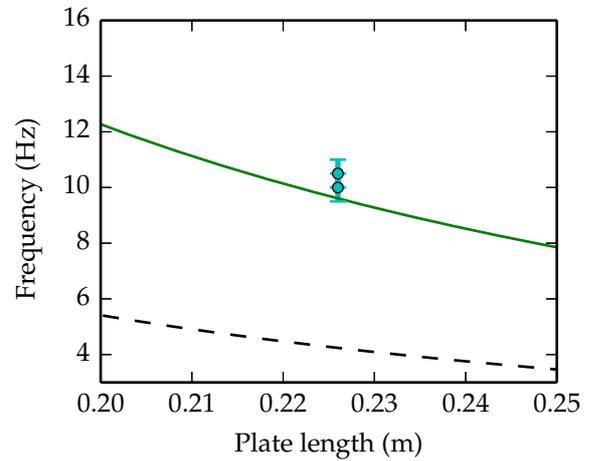
**FIGURE 5.** Characterization of boundary conditions. Blue dots: experimental points, solid line: theoretical values in a clamped-clamped configuration, dotted line: theoretical values in a pinned-pinned configuration.
