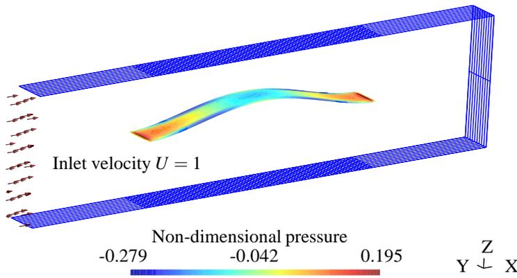
of the plate, showing that 3D effects occur near the lateral edges of the plate. Both ends of the plate are a singularity for the fluid; therefore the pressure distribution is truncated before the numerical discrete expansion on the natural modes basis.
