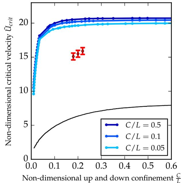
**FIGURE 8.** Evolution of the dimensionless critical velocity with lateral confinement for  $\frac{D}{L} = 0.05, 0.1, 0.5$ . Blue lines: numerical simulations. Red dots: experimental values. Black line: reference model (see [1]).
