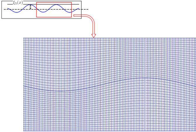
**FIGURE 2.** Detail of the mesh generated in the fluid domain near the plate deformed with a 5<sup>th</sup> mode shape  $\xi_5(x)$
