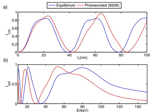
FIG. 6: Results of dynamical diffraction theory including  $N = 26$  beams. a) Intensity of the (220) peak at the Bragg angle,  $I_{220}(s = 0)$  for varying sample thicknesses, assuming 45 keV electrons. b) Intensity of the (220) peak at the Bragg angle,  $I_{220}(s = 0)$  for varying electron energy, assuming a 70 nm thickness.
