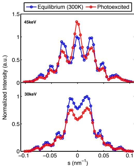
FIG. 4: Top: experimental rocking curves for the (2-20) peak taken with 45 keV electrons, at equilibrium  $T = 300$  K (blue curve) and in the photo-excited state (red curve), taken at  $t = 150$  ps delay. Bottom: same but using 30 keV electrons as a probe. The rocking curves were normalized relative to the equilibrium case.
