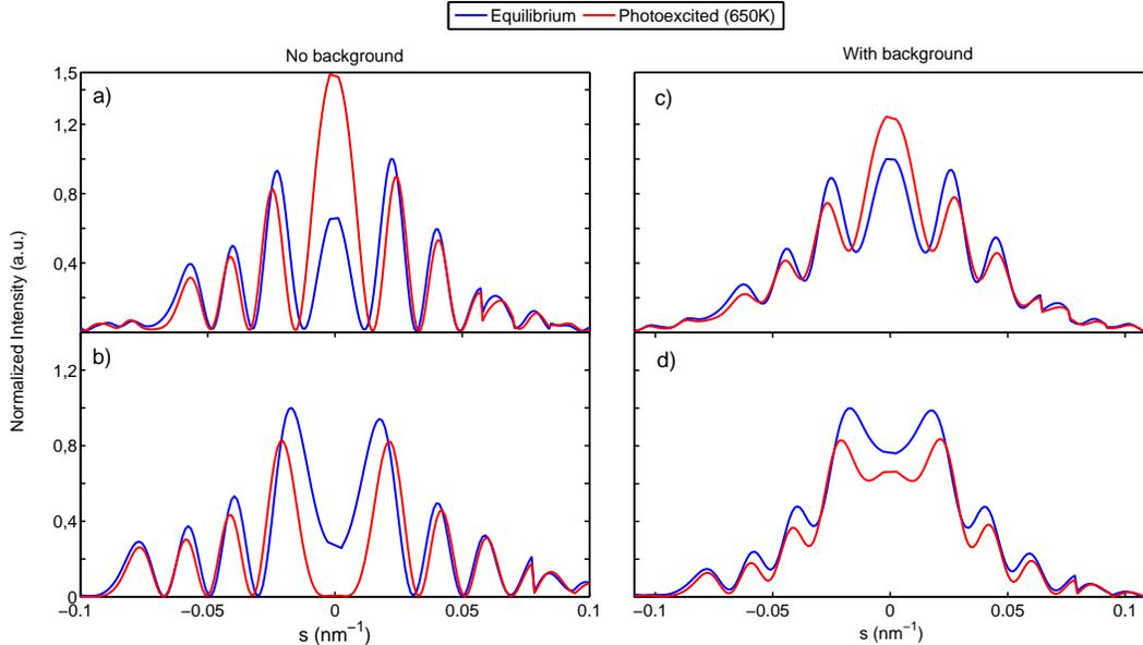
FIG. 5: Results of N-beam dynamical diffraction theory with  $N = 26$  beams: a) calculated rocking curves for the (2-20) peak in the case of 45 keV electrons. The blue curve shows the result at  $T = 300$  K and at  $T = 650$  K (red curve), b) same calculations but with 30 keV electrons. In figures c) and d), a gaussian background that was added to the N-beam calculations in order to better fit the data. The rocking curves are normalized relative to the equilibrium case.
