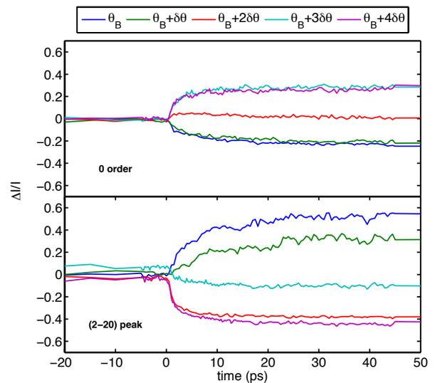
FIG. 3: Photo-induced dynamics for various sample orientations. The blue curve is obtained when the sample is exactly at the Bragg angle; the other curves are obtained by tilting the sample by  $\delta\theta = 0.26^\circ$ . The incident fluence is  $12 \text{ mJ/cm}^2$ . Top: dynamics of the transmitted beam. Bottom: dynamics of the (2-20) peak.
