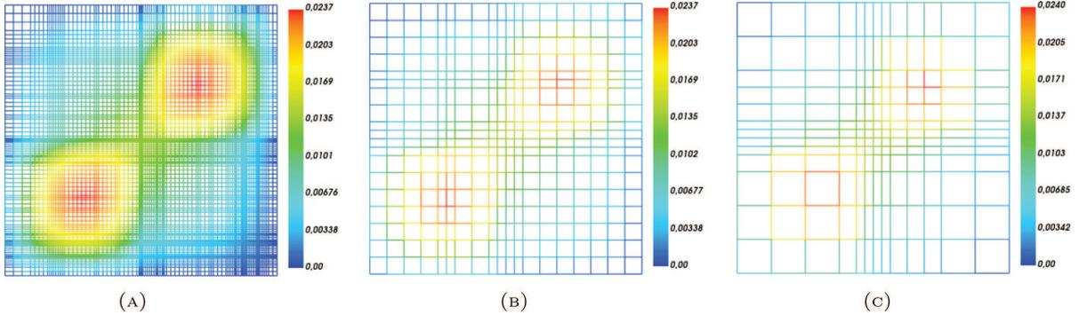
FIGURE 7. The numerical flux  $\phi_h$  for different reconstruction methods. (A) Average reconstruction (5.1). (B) *Reconstruction* associated to the RTN post-processing (5.6). (C) *Reconstruction* associated to the  $RTN_0$  post-processing (5.3).
