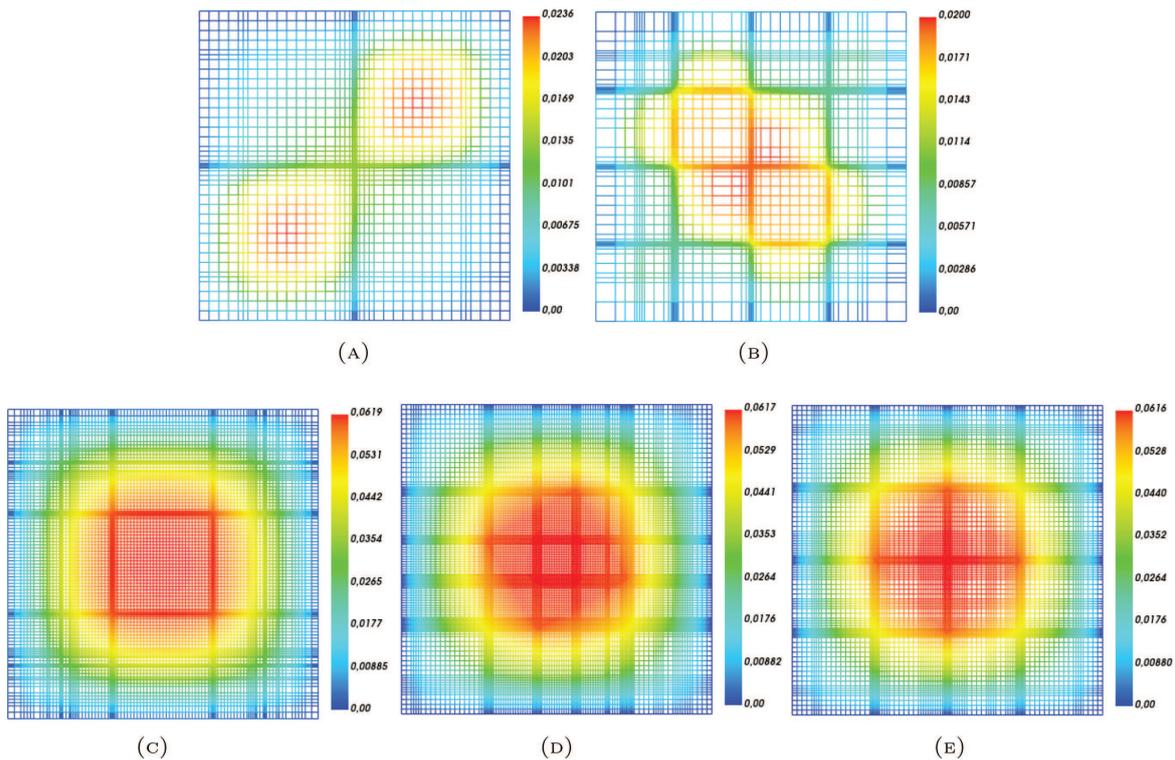
FIGURE 5. The numerical flux  $\phi_h$  of the optimal threshold value for the different test cases. (A) Dauge,  $\theta_l = 0.35$ . (B) Checkerboard,  $\theta_l = 0.35$ . (C) Center,  $\theta_l = 0.6$ . (D) Rotation Center,  $\alpha = \pi/6$ ,  $\theta_l = 0.45$ . (E) Rotation Center,  $\alpha = \pi/4$ ,  $\theta_l = 0.4$ .
