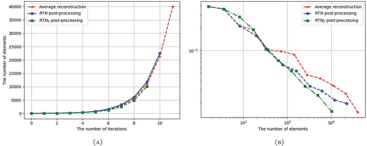
FIGURE 8. Evolution of the number of elements and the relative  $L^2$  error (6.4) for different reconstruction methods : namely the *average reconstruction* (5.1), the *reconstruction* associated to the RTN post-processing (5.6) and the *reconstruction* associated to the  $RTN_0$  post-processing (5.3). (A) Number of elements. (B) Relative  $L^2$  error.
