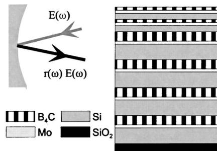
Fig. 1. Aperiodic multilayer structure of the three-material broadband XUV mirror. From the top to the bottom, there are two 16.3 nm thick and four 40.6 nm thick B<sub>4</sub>C/Mo/Si layers sitting on a SiO<sub>2</sub> substrate.
