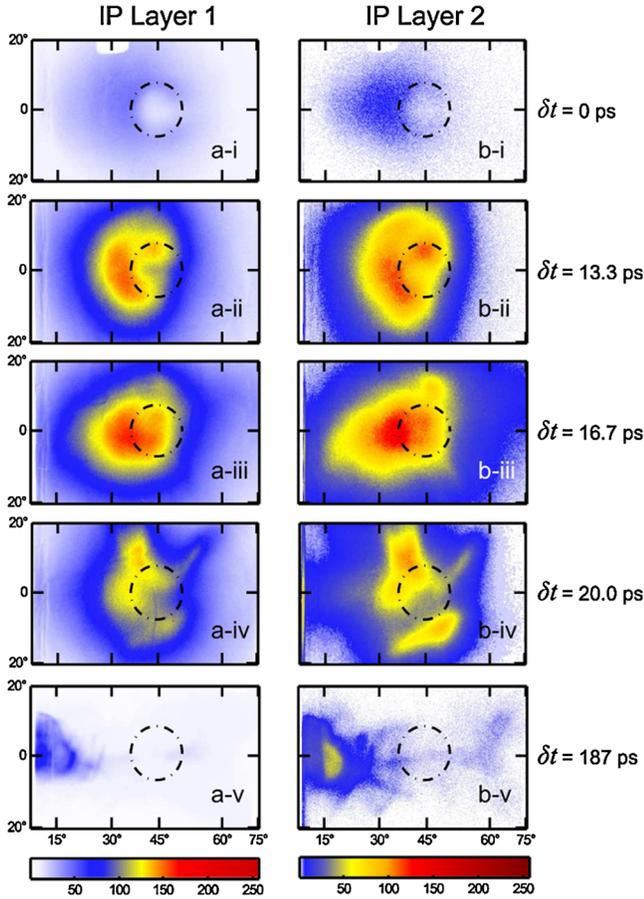
FIG. 2 (color online). Single-shot exposures of the electron beam from SiO<sub>2</sub> plasma for different prepulse delays ( $\delta t = 0, 13.3, 16.7, 20.0$  and  $187$  ps). The laser intensity is  $2.5 \times 10^{18}$  W/cm<sup>2</sup> incident along the 45° angle (marked with a dotted circle); the target surface direction is along the 90° angle). The left and right columns show electrons registered on IP layer 1 (>150 keV) and layer 2 (>350 keV), respectively.
