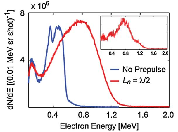
FIG. 3 (color online). Electron spectra measured along the  $\phi = 36^\circ$  direction by accumulating 250 laser shots at  $I \sim 2 \times 10^{18}$  W/cm<sup>2</sup> for the case of no prepulse [blue (dark gray)], and a scale length of  $\approx \lambda/2$  [red (medium gray)]. The inset shows the spectrum from a single laser shot for the optimal scale length of  $\sim \lambda/2$ .
