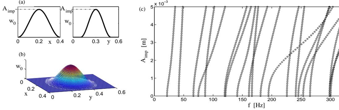
Figure 12: (a): cross-section (in the  $x$  and  $y$  directions) of the imperfection of amplitude  $A_{imp}$  (in m) considered for the plate. (b): three-dimensional view of the imperfect plate. (c) : eigenfrequencies (in Hz) for increasing values of  $A_{imp}$ .
