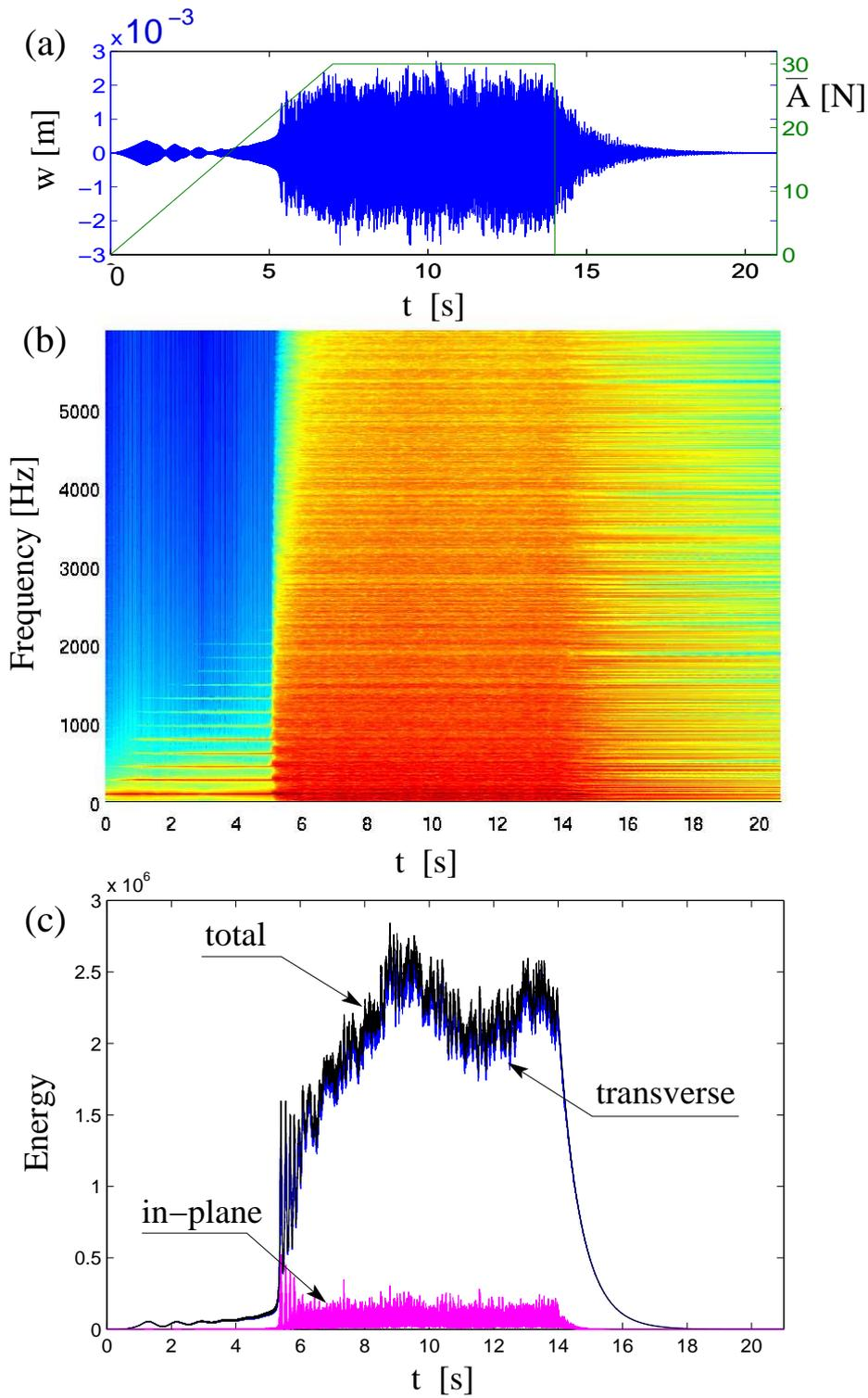
Figure 4: Transverse vibration and energy of the damped plate ( $\sigma_0=0.75$ ) excited at 87 Hz. (a): output transverse displacement  $w^{out}$  and history of the loading amplitude  $\bar{A}$ . (b): Spectrogram of  $w^{out}$ . (c): Total discrete energy  $h$  (black) of the plate during the simulation: transverse component  $t + v$  (blue) and in-plane component  $u$  (magenta).
