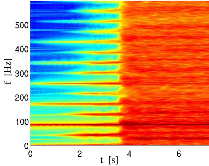
Figure 13: Spectrogram of output for the imperfect plate excited at 85.5 Hz, with a forcing amplitude  $F$  from 0 to 60 N in 20 seconds (with only the first 8 seconds shown). A clear 1:2 internal resonance is excited for  $F=4$  N before the turbulent regime sets in for  $F=12$  N.
