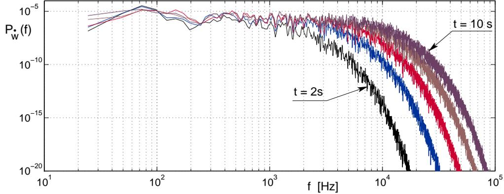
Figure 17: Power spectra of the velocity, for the simulation with  $f_S = 400$  kHz, and at successive instants, respectively:  $t = 2$  s, 4 s, 6 s, 8 s and 10 s. Power spectra are compute with windows of 16384 points (0.041 s), mean-valued over twelve successive windows so that 0.5 seconds of signal is used at each instant.
