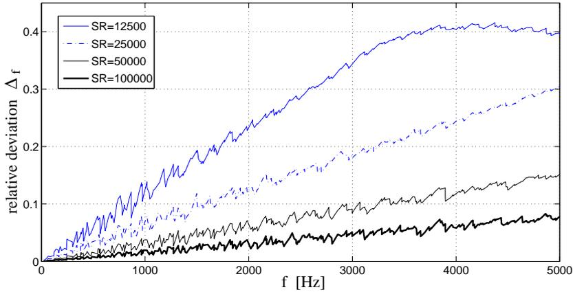
Figure 2: Relative deviation  $\Delta_f^i$  between analytical eigenfrequencies of a simply supported plate and those computed with the finite difference scheme with increasing  $f_s$ , in the frequency range  $[0, 5000]$  Hz.
