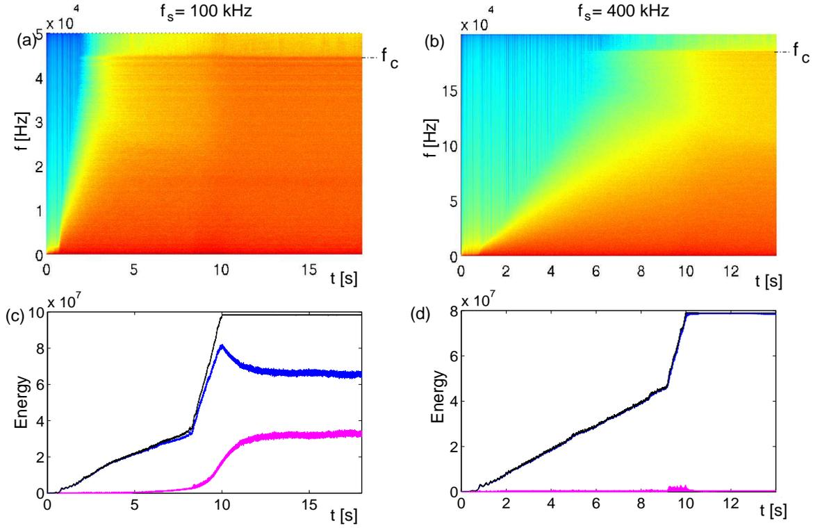
Figure 16: Spectrograms and Energies for the undamped plate excited at  $f^{exc} = 75$  Hz. (a)-(c):  $f_s = 100$  kHz, (b)-(d):  $f_s = 400$  kHz. Bending energy in blue, in-plane energy in magenta, total energy in black.
