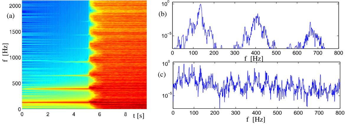
Figure 8: (a): Spectrogram of the output vibration  $w^{out}$  for the plate excited at 130 Hz, with a forcing amplitude  $F$  from 0 to 30 N in 10 seconds. A direct transition is observed with frequency peaks of increasing width just before the turbulent regime. (b) and (c) : Fourier transforms of a 1.3 sec segment computed respectively at  $t=5$  s and  $t=8$  s.
