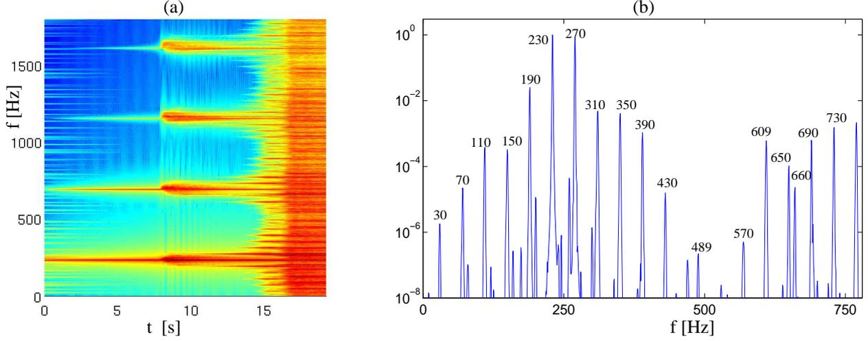
Figure 11: (a): Spectrogram of the vibration  $w^{out}$  for the perfect plate excited at 230 Hz, with a forcing amplitude  $F$  from 0 to 110 N in 20 seconds. (b): Fourier transform of 1.3 sec of the displacement at  $t=15$  s.
