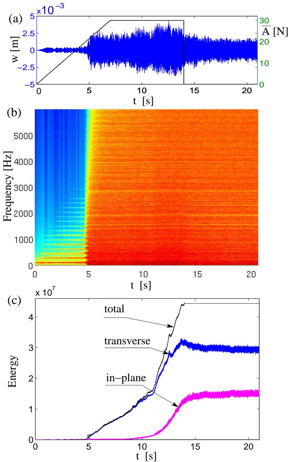
Figure 3: Transverse vibration and energy of an undamped plate excited at 87 Hz. (a): transverse displacement  $w^{out}$  at one point on the plate and history of the dimensioned loading amplitude  $\bar{A}$  on the right axis. (b): Spectrogram of  $w^{out}$ . (c): Total discrete energy (arbitrary units)  $\eta$  (black) of the plate during the simulation, decomposed into its bending (transverse) component  $t + v$  (blue) and its in-plane component  $u$  (magenta).
