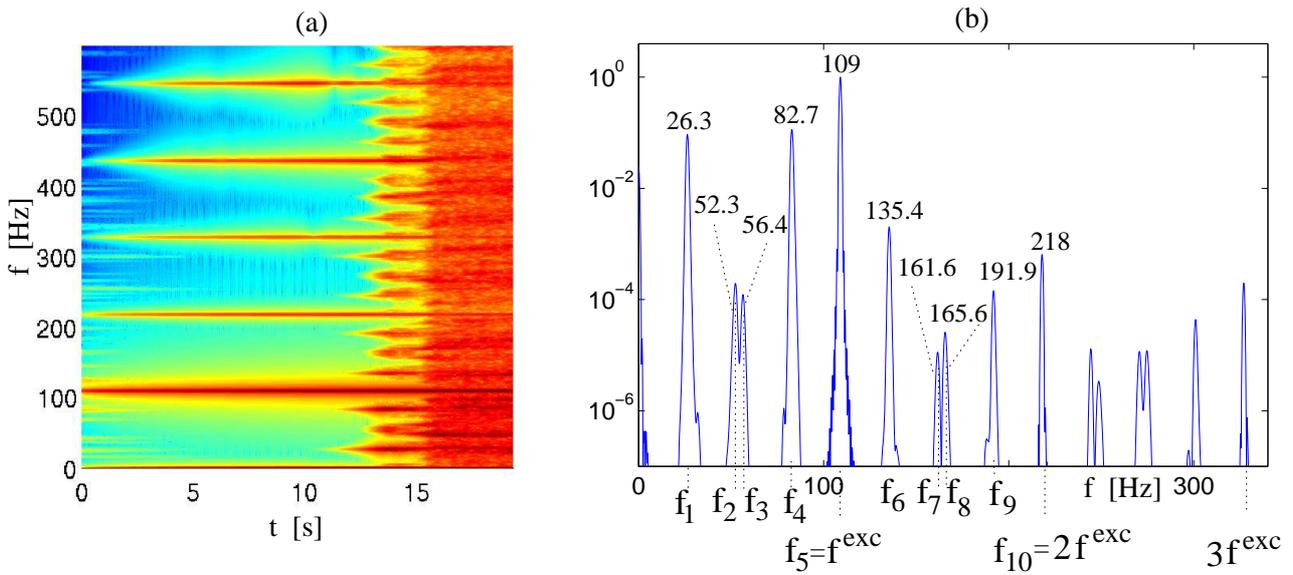
Figure 14: (a) Spectrogram of output for the imperfect plate excited at 109 Hz, with a forcing amplitude  $F$  from 0 to 50 N in 20 seconds. (b) Fourier transform of 1.3 sec of the displacement  $w^{out}$  at  $t=14$  s, showing the combination resonances before the turbulent behaviour.
