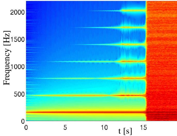
Figure 5: Spectrogram of output displacement  $w^{out}$  for the plate excited at 154 Hz, with a linearly increasing force from 0 to 60 N over 20 seconds. A direct transition to turbulence is observed, occurring at  $t=15$  s, *i.e.* for  $F=45$  N.
