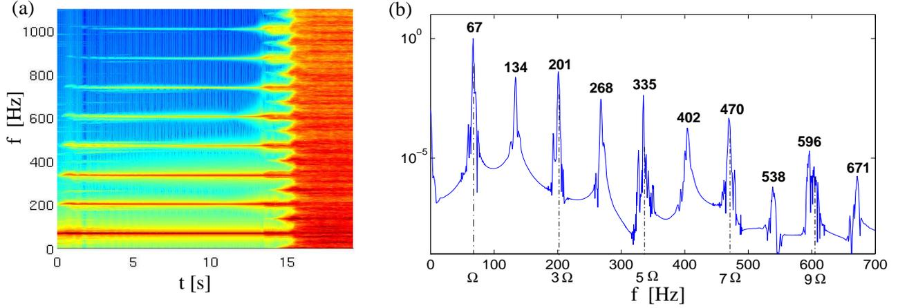
Figure 7: (a): Spectrogram of output vibration  $w^{out}$  for the plate excited at 67 Hz, with a forcing amplitude  $F$  from 0 to 50 N in 20 seconds. A symmetry-breaking (SB) bifurcation is observed with the appearance of even harmonics in the response, before the turbulent regime. (b): Fourier transform of a 1.3 sec segment (Hanning window of  $2^{16}=65536$  points) computed at  $t=14.5$  s showing the spectral content of the vibration after the SB bifurcation.
