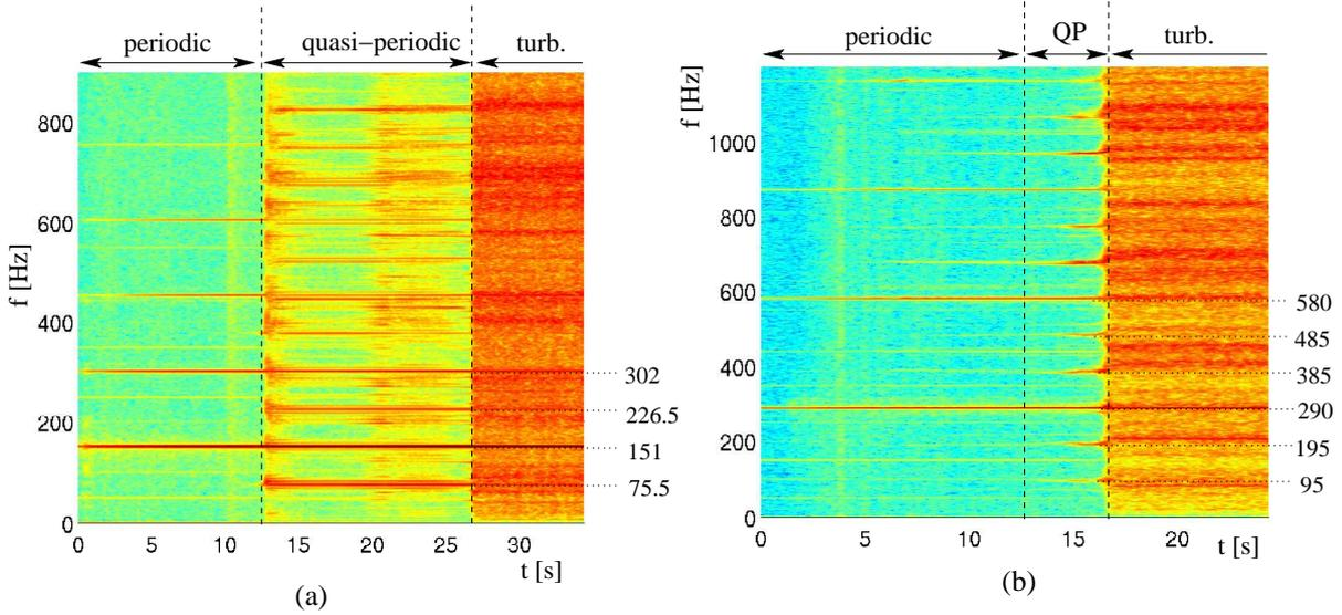
Figure 1: Experimental spectrograms of the vibration velocity for a rectangular plate excited with a harmonic force of increasing amplitude and frequency 151 Hz (a), and 290 Hz (b). In each case the three different vibration regimes are clearly identified.
