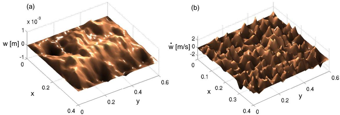
Figure 15: (a) Transverse displacement of the plate  $w(x, y)$  in the turbulent regime. (b) Transverse velocity  $\dot{w}(x, y)$ . The undamped plate is excited at  $f^{exc}=87$  Hz with a forcing amplitude  $\bar{A}=30$  N.
