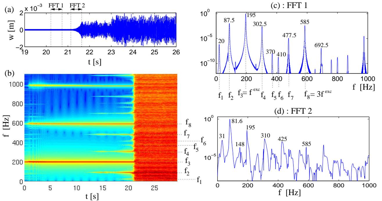
Figure 10: Transition scenario to turbulence for the perfect plate excited at 195 Hz, with a forcing amplitude from 0 to 35 N in 30 seconds. (a) : time series of the output displacement  $w^{out}$ , zoom on the transition between 19 and 26 s. (b) : spectrogram of the vibration. (c) and (d) : Fourier transforms of 0.65 s of the displacement, respectively at  $t=20$  s (c), and  $t=21.1$  s (d).
