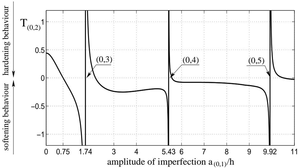
Figure 5: Type of non-linearity for mode (0,2) with an axisymmetric imperfection having the shape of mode (0,1). 2:1 internal resonances with modes (0,3), (0,4) and (0,5) occurs respectively for  $a_{(0,1)}/h = 1.74, 5.43$  and  $9.92$ .
