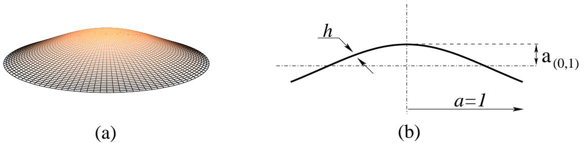
Figure 2: (a) Three-dimensional view and (b) cross-section of the circular plate with geometric imperfection having the shape of the first axisymmetric mode. As non-dimensional quantities are used,  $a = 1$  and the amplitude  $a_{(0,1)}$  of the imperfection is made non-dimensional with respect to the thickness  $h$ .
