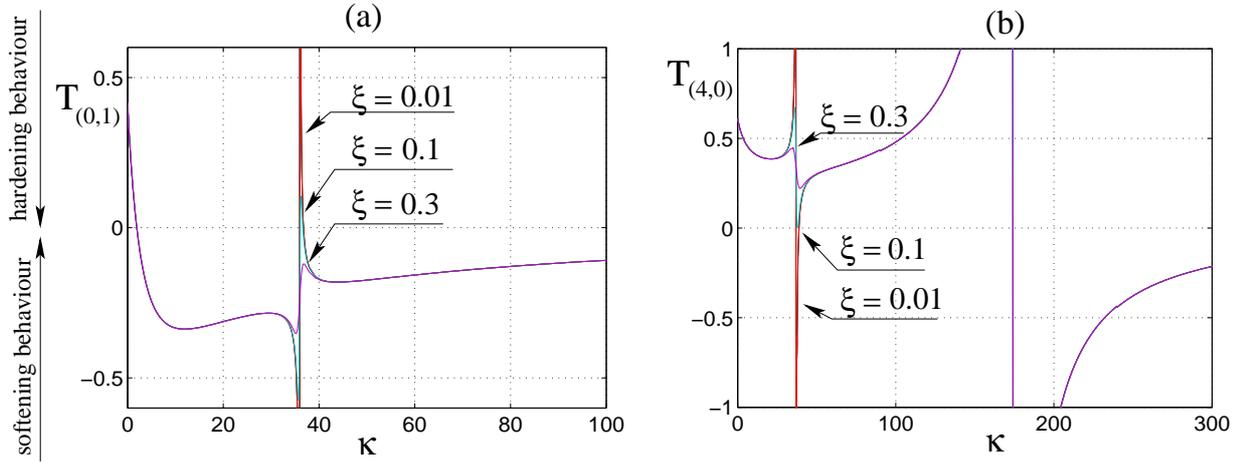
Figure 11: Type of non-linearity for (a): mode (0,1) and (b): (4,0) versus the aspect ratio  $\kappa$  of a shallow spherical shell. Increasing values of damping for case (i) ( $\forall p = 1 \dots N, \xi_p = \xi / \omega_p$ ), are shown, with  $\xi = 0$  and 0.01 (red), 0.1 (cyan) and 0.3 (violet).
