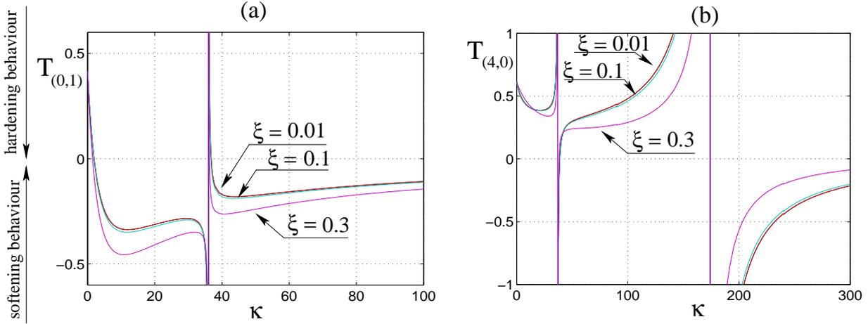
Figure 12: Type of non-linearity for (a): mode (0,1) and (b): (4,0) versus the aspect ratio  $\kappa$ . Increasing values of damping for case (ii) ( $\forall p = 1 \dots N, \xi_p = \xi$ ), are shown, with  $\xi = 0$  and 0.01 (red), 0.1 (cyan) and 0.3 (violet).
