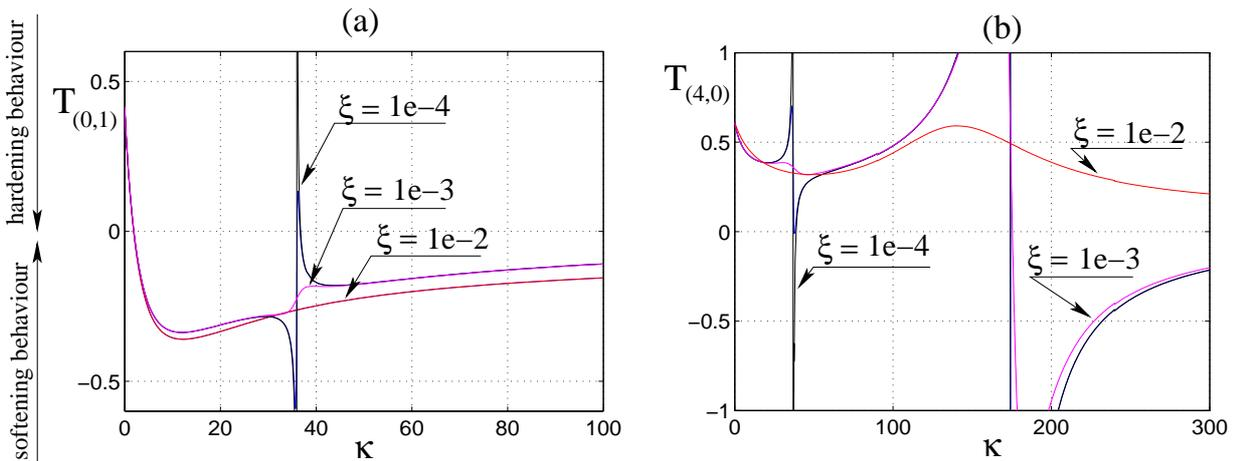
Figure 13: Type of non-linearity for (a): mode (0,1) and (b): (4,0) versus the aspect ratio  $\kappa$ . Increasing values of damping for case (iii) ( $\forall p = 1 \dots N, \xi_p = \xi \omega_p$ ), are shown, with  $\xi = 0$  and 1e-4 (black), 1e-3 (magenta) and 1e-2 (red).
