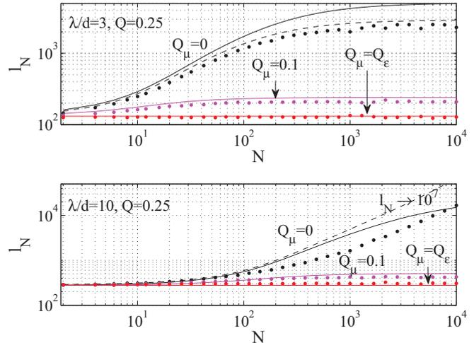
FIG. 4. (Color online) Attenuation length  $l_N$  of a mixed stack as a function of  $N$  for  $\lambda/d = 3$  and  $\lambda/d = 10$ . Same convention as in Fig. 3 is used. The transition starts for  $N = 1/Q^2(kd)^2$  ( $N \sim 4$  for  $\lambda/d = 3$  and  $N \sim 40$  for  $\lambda/d = 10$ ). For  $\lambda/d = 10$ ,  $Q_\mu = 0$ , the asymptotic  $l_N = L_{\text{loc}} \sim 10^7$  is found from Refs. 6 and 7 for  $N > 10^7$ .
