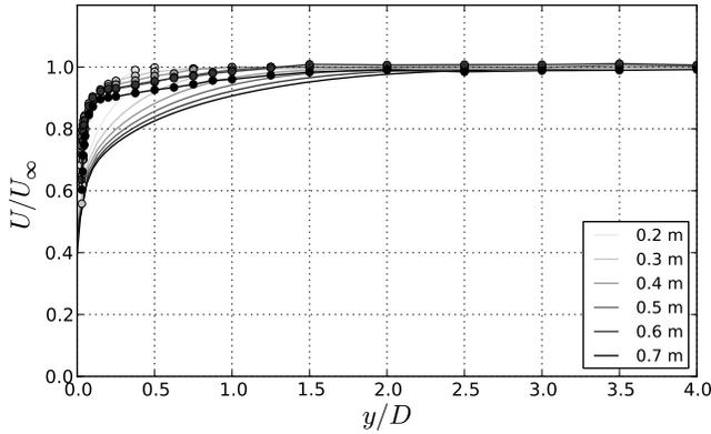
**FIGURE 7.** VELOCITY PROFILES: • EXPERIMENTS AND – CFD SIMULATIONS
