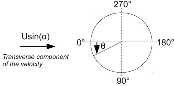
**FIGURE 10.** ANGULAR POSITION OF THE PRESSURE TAP
