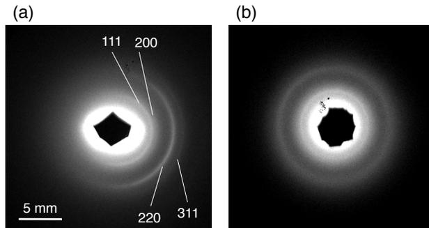
FIG. 3: Electron diffraction patterns from a 10 nm thick polycrystalline Al foil. (a) The diffraction pattern is asymmetric because of a spatial chirp in the electron beam. (b) Symmetric diffraction pattern obtained by removing the spatial chirp on the electron beam.
