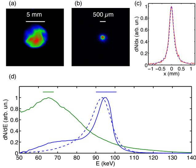
FIG. 2: (a) Unfocused beam after filtering through a 1 mm pinhole. (b) Best focus obtained using the solenoid. The FWHM is  $D = 280 \mu\text{m}$ . (c) Horizontal lineout of the beam profile (red curve) and GPT simulation results (blue curve). (d) Normalized electron distribution of the unfocused beam (green curve), focused beam (blue curve) and simulation results of the focused beam (dashed blue curve). The top error bars represent the resolution of the spectrometer at various energies.
