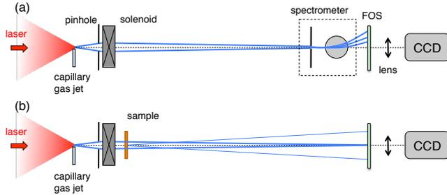
FIG. 1: (a) Experimental set-up for electron beam characterization with an electron spectrometer. (b) Set-up for diffraction. The solenoid is placed 60 mm after the electron source, the distance between the sample and the scintillator (FOS) is 220 mm.
