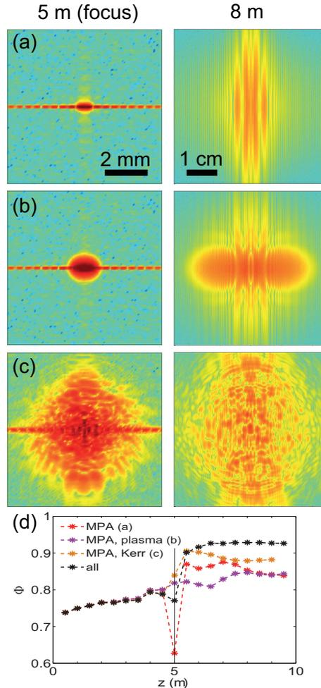
FIG. 6. Influence of the different nonlinear terms. (a)-(c) Beam profiles at  $z = 5, 8 \text{ m}$  from numerical results corresponding to simulations with identical conditions as in Fig. 5: (a)  $n_2, \sigma = 0$ , (b)  $n_2 = 0$ , (c)  $\sigma = 0$ . Color scale is that of Fig. 5. (d) Evolution of symmetry degree for (a)-(c) and Fig. 5. The nonlinear effects that are *on* in each simulation are listed in the legend.
