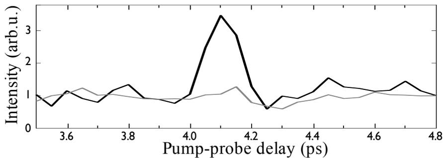
**Figure 6.** Pump-probe scan in a 50/50 mixture of nitrogen and argon. The black line was obtained with polarization resolved pump probe spectroscopy while the grey line was obtained with conventional detection.
