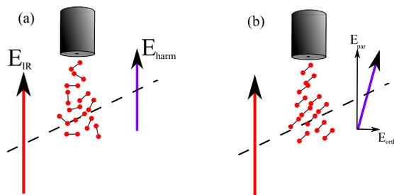
**Figure 4.** Principle of polarization resolved spectroscopy. In an isotropic medium, the harmonic polarization is parallel to the laser field (a). In an anisotropic medium this is in general not the case and an orthogonal electric field component can be produced (b).
