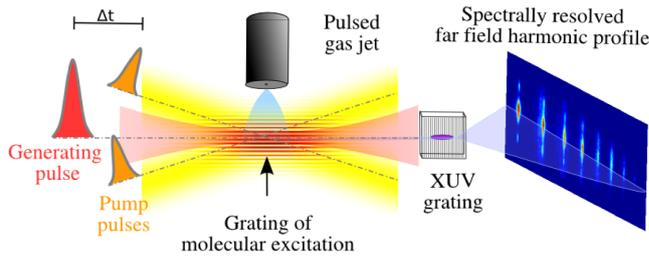
**Figure 1.** Experimental setup for high harmonic transient grating spectroscopy. Two crossed pump pulses create a grating of rotational excitation. A delayed probe pulse generates high harmonics in the excited medium. The emitted light is analyzed by an XUV spectrometer that images the spatial profile of each harmonic.
