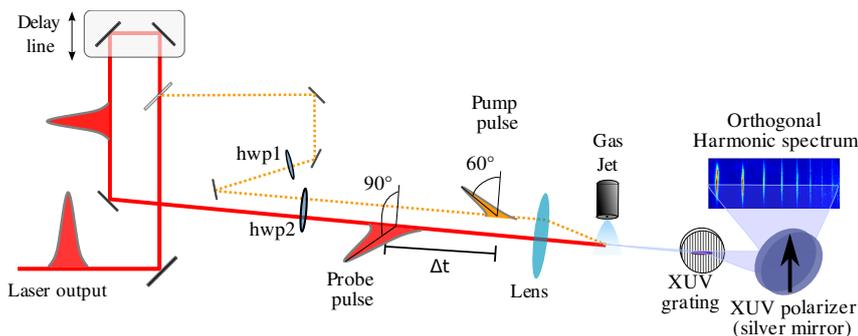
**Figure 5.** Experimental setup for polarization resolved pump probe spectroscopy. The probe beam polarization is orthogonal to the polarizer axis. The pump beam polarization is in between, so that symmetry is broken when molecules are aligned.
