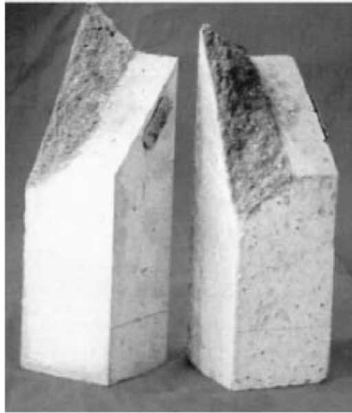
Fig. 36. Experimental crack path from [89].
