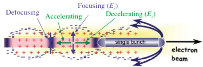
**Figure 1.** Concept of the PWFA using a *single* drive bunch. Note: for clarity, the transverse and longitudinal fields are indicated in second bucket but have the same signs and relative locations in all buckets.
