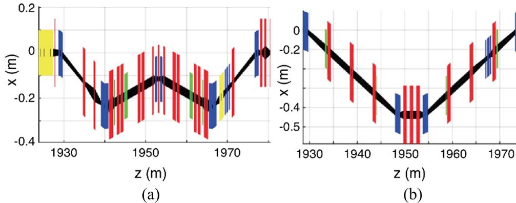
**Figure 5.** Existing final electron compression chicane (a) and its redesigned version with fewer magnets (b). Quadrupole magnets are shown in red, bends are in blue, sextupoles are in green. The yellow boxes in (a) show the accelerating structures at the end of the linac and the transverse cavity (the so-called T-CAV, essentially an  $x$ -band ‘streak camera’) in the chicane. For the re-designed optics, the transverse cavity is included in the beamline downstream of the chicane.
