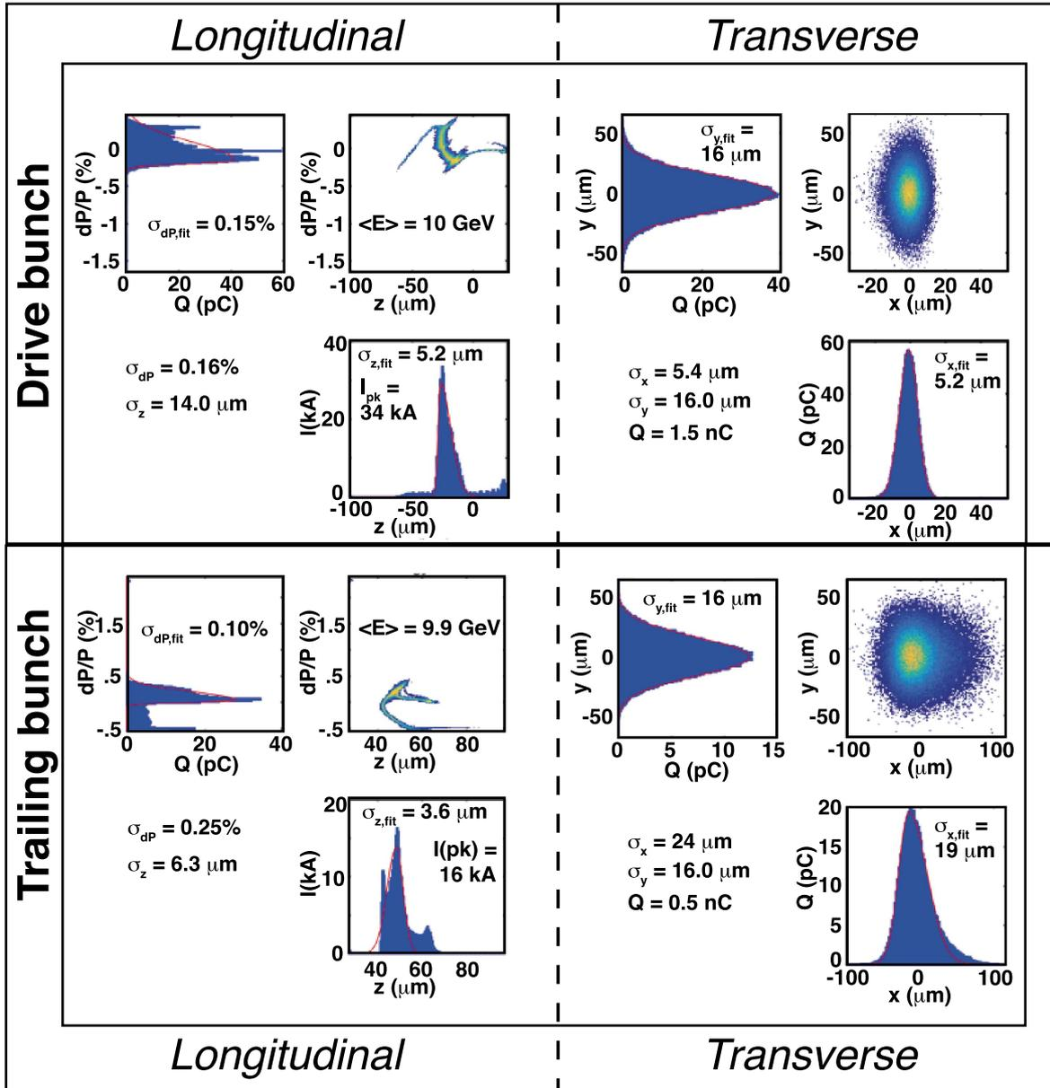
**Figure 6.** Results of 6D particle tracking, shown at the interaction point (IP), after tracking the particles from the RF gun to the IP (entrance to the plasma). Drive (witness) beams have  $x$  by  $y$  emittances of  $7.2 \times 3.2$   $\mu\text{m}$  ( $7.4 \times 3.0$   $\mu\text{m}$ ) which, for this simulation, have about twice the peak current in both bunches with respect to the minimum performance initially requested by PWSA experimentalist via 3D PIC simulations (see table 1).
