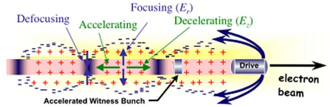
**Figure 2.** Concept of the PWFA using *separate* drive and witness bunches. Note: for clarity, the transverse and longitudinal fields are indicated in second bucket but have the same signs and relative locations in the all buckets.
