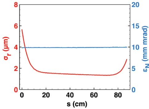
**Figure 10.** Beam spot size variation (red curve) and the emittance variation (blue line) throughout the plasma with matching sections. Values are full projections of the trailing bunch. The vacuum waist size occurs at  $s = 0$  cm and the injected bunch has a normalized emittance of  $10 \mu\text{m}$ .
