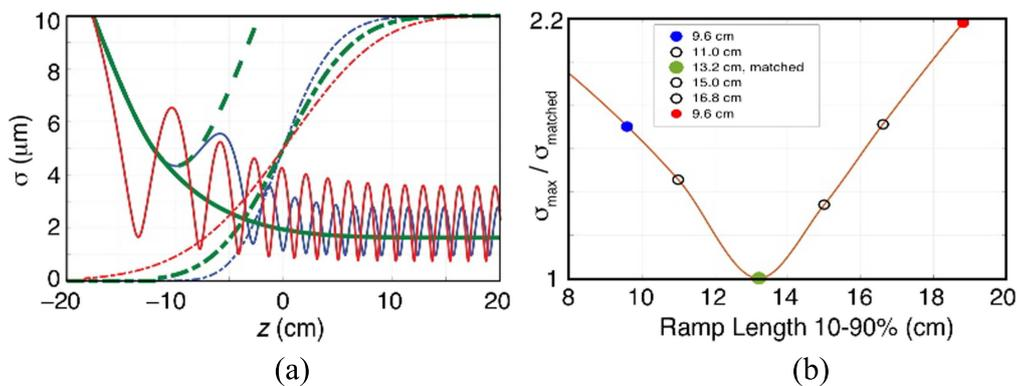
**Figure 9.** (a) An example of the determination of incoming beam parameters to match a particular profile (heavy green lines, see text) and the betatron oscillations of that same incoming beam if the profile were to change (red and dark-blue lines). (b) A summary of the maximum betatron spot size within the plasma normalized to the matched size for six profiles, three of which are shown in (a).
