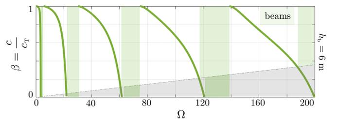
FIG. 3: Dispersion of elastic SPPs, from (9) with out-of-plane motion for  $h_b = 6$  m. Intrinsic band-gaps are opened due to flexural resonances (light green regions outside of the Brillouin zone) which are enlarged by periodicity (light green regions inside the Brillouin zone).
