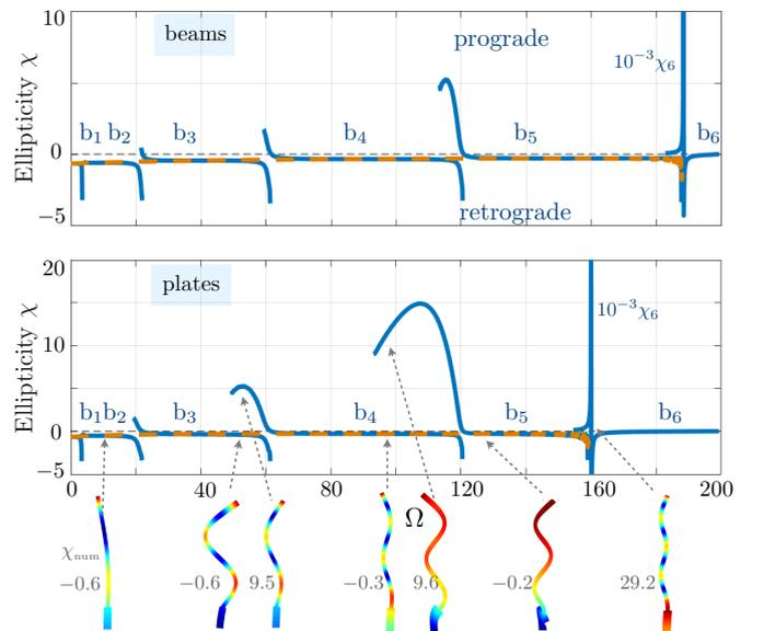
FIG. 5: Ellipticity  $\chi$  of the hybridized Rayleigh waves versus  $\Omega$  for beams (upper panel) and for plates – Blue lines show  $\chi$  from (10), dashed red lines neglecting the flexion ( $f_F = 0$  in (10)). Insets show the deformations in the plates atop the soil in a single cell, computed numerically and the corresponding ellipticity  $\chi_{\text{num}}$  (see main text).
