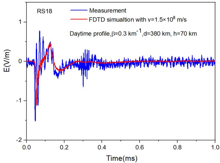
Fig. 12. Comparison between the FDTD simulation and experimental data for the negative return stroke labeled RS18 (in Fig. 3a) of the bipolar flash of 21 September 2014, 15:14:09 (local time).
