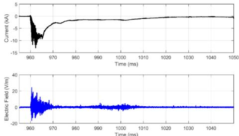
Figure 1. Current (top) and E-field (bottom) waveforms associated with a type-2 upward positive flash that occurred on 21<sup>th</sup> October 2014, 23:56:46 (local time).
