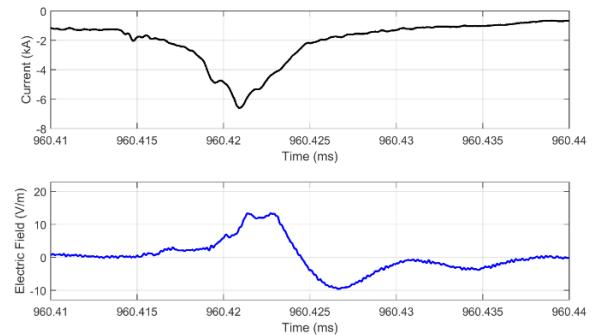
Figure 2. The first category of observed pulses (Category A pulse). Current (top) and electric field (bottom). The overall flash waveforms are shown in Figure 1.
