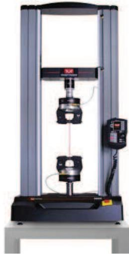
FIGURE 5.18: La machine de traction INSTRON
