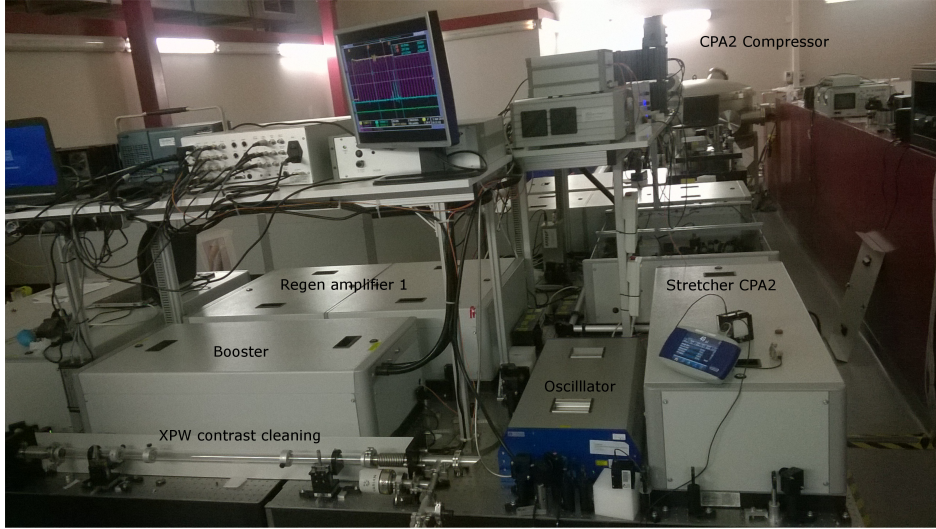
Figure 4.1 – 200 TW SAPHIR laser system in upgraded contrast configuration in 2016
